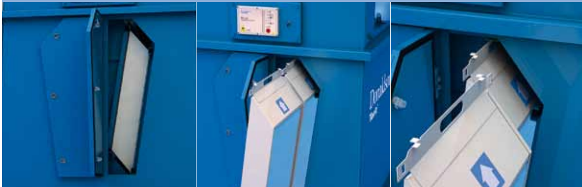
Open filter access doors. (Clean side of the system)
